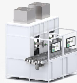
MICRO.SPECTOR Inline microscopic inspection
