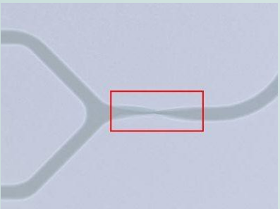
thin spots & lamination issues
